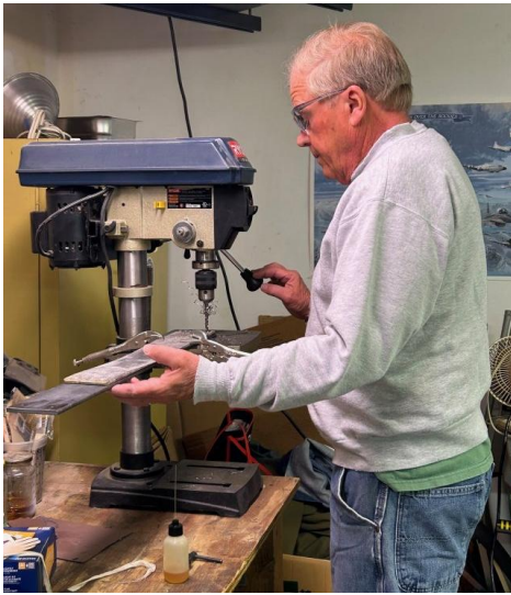
Mark Palmer drills holes for 840's new skid plates (spoiler alert: he's really not that tall).
