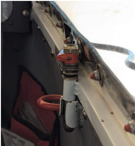
2-33 canopy latched as viewed from the back seat. Photo by Jon Stark
