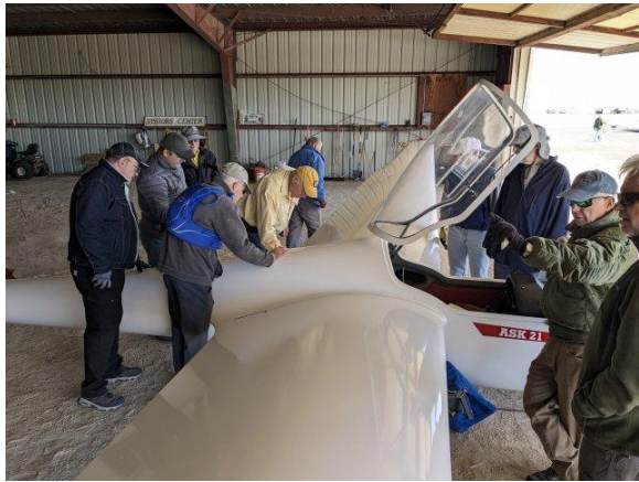
The drag spar pins took a bit of fiddling. Photo by Todd Hahn
