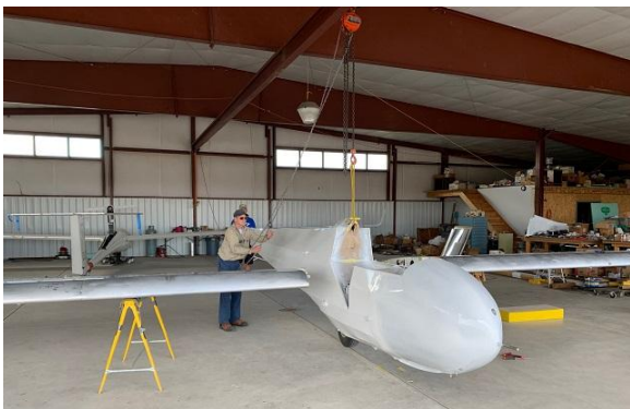
Doug hoists the fuselage in preparation for mating the wings to fuselage. Photo by John Gillis.
