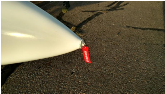
Frank's solution: a $2.50 rubber sink plug and a "Remove Before Flight" lanyard.
