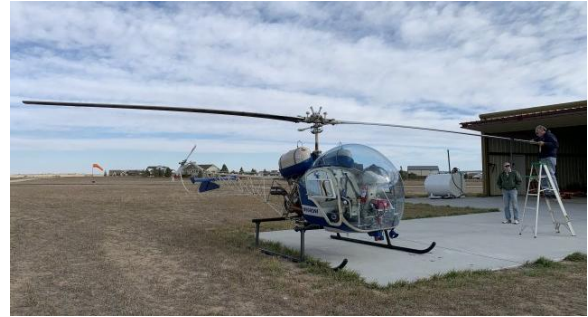
At long last, Jon Stark gets ready to fly his Bell 47. Helicopter mechanic Paul McKenzie is balancing one of the blades.
