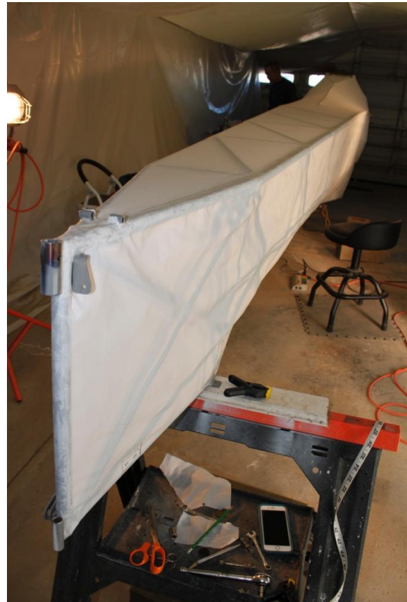
Bottom and left side fabric is glued (fuselage is upside down)
