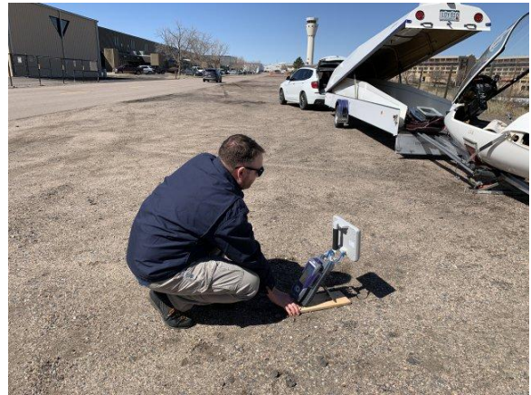
Bradley Parsons of Arapahoe Aero conducts a transponder check on Raul Boerner's LS-6.
