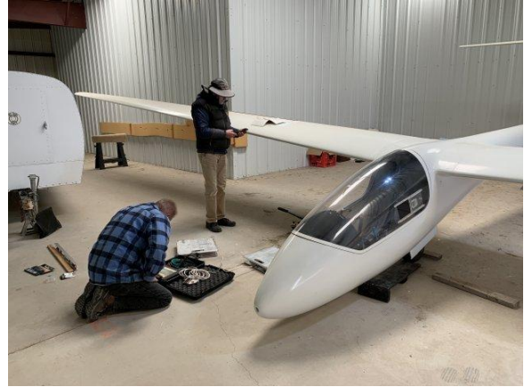
Jamie Treat sets up to do a weight and balance on Jon Stark's Phoebus, ONE.
