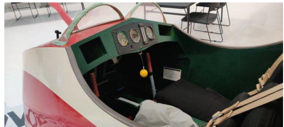
Cockpit of the T.21. Note the pellet vario. Photo by Vitaliy Aksyonov
