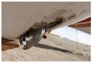
Cracked nose cone area and tired tow hook
