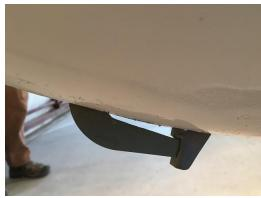
New tow hook installed after nose cone repairs
