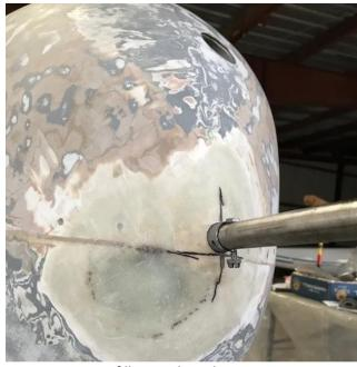
Nose cone filling and sanding in progress
