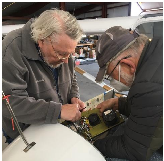
Dave and Gary work on the instrument panel electrical connections.
