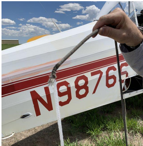
The rest of the line. About three feet of sheathing had been removed.
