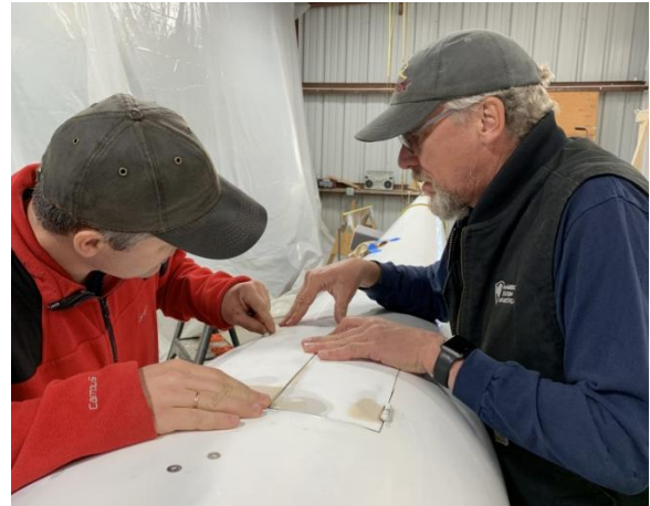
Vitaliy Aksyonov and John Gillis fit the newly rebuilt gear doors on the Russia, 87E.
