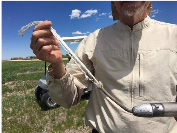
Here you can see the sheathing on the line was stripped away as the takeoff roll began. The line has already been cut at this point to begin the repair.
