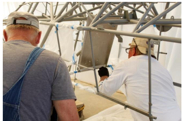
Mark strips the old paint from the seat back, with assistance from Gary
