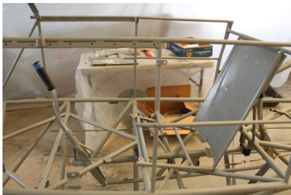
Elevator controls going back in
