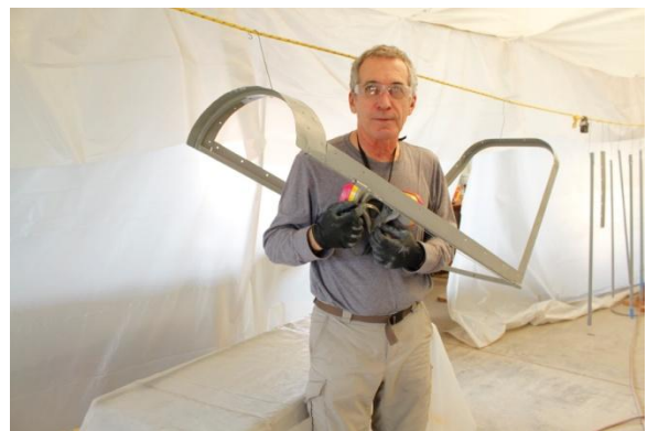
Raul invested lots of elbow grease cleaning up the rusty canopy frame before priming
