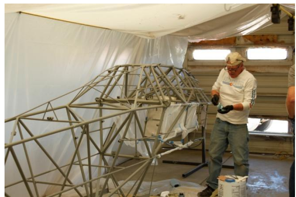
Doug's invaluable fuselage stands allow complete fuselage rotation
