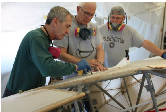
Raul, Frank, and Gary install gussets.
