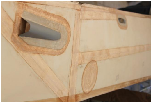
Elevator and rudder fairleads and inspection ring with gussets installed.
