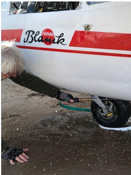
Wojciech Tomanek hoses out the Blanik wheel well. The landing gear system on the L-23 is a very efficient mud scoop. Photo by Raul Boerner
