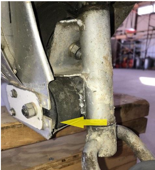
Separation of the tailwheel shock absorber
