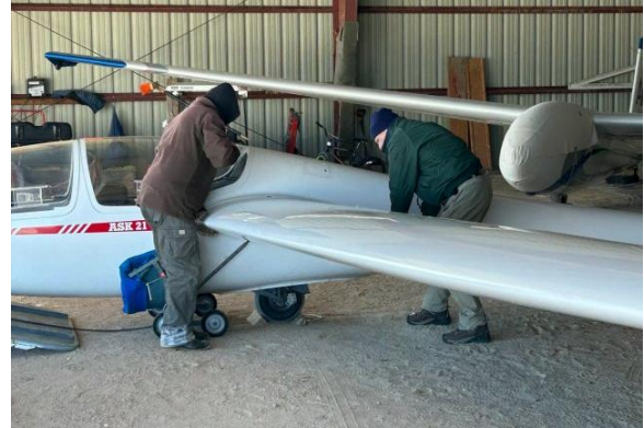
Bill Gerblick and Colin Mead remove the left wing. Photo by Doug Houston
