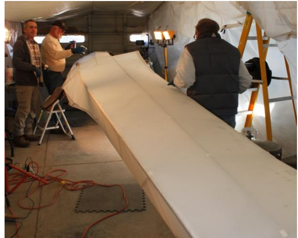
Heat shrinking is complete.
