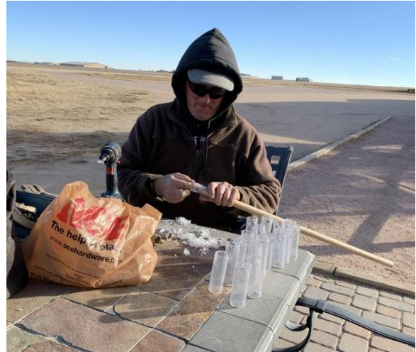
What do towpilots do at the end of the day when the sun's still out? Bill Gerblich makes a bunch of replacement vinyl sleeves for the towline bullets.
