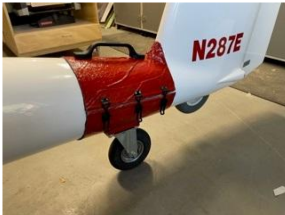
The Russia's new tail dolly (more pictures at the end of this issue)
