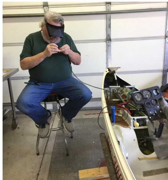
The Mad Tinkerer, Dave Rolley, rewires the Palmer’s transponder cable.
