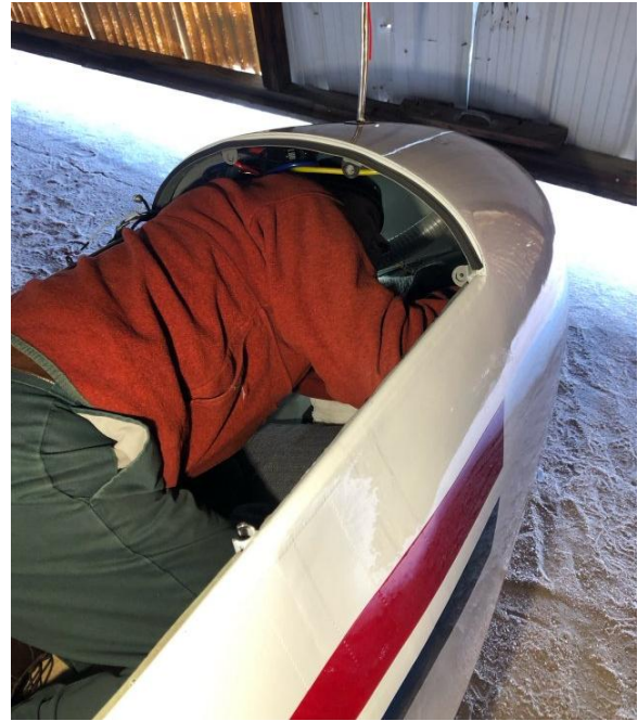
Doug Curry installing the transponder antenna in 840. Photo by Bill Gerblich
