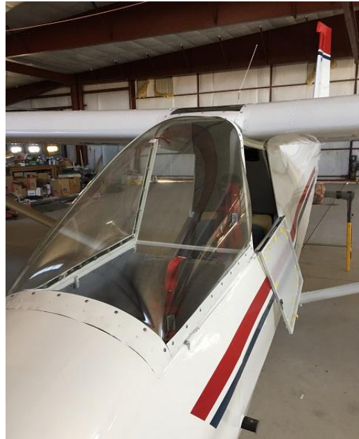
Canopy and window installed
