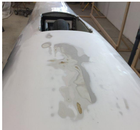
Vitaliy sanded down the rough spots.
