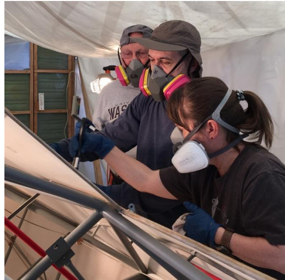
Gary, Raul, and Becky apply a finishing tape.
