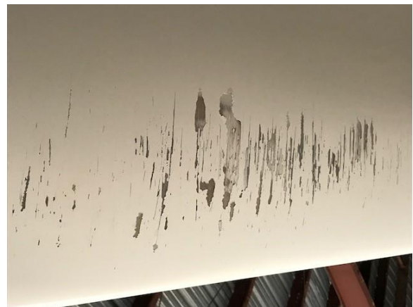
The results of dragging the ASK wing over the rocks
